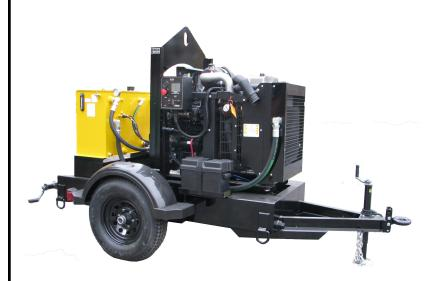
This model features a John Deere 4 cylinder water cooled diesel with your choice of fixed displacement gear or pressure compensated piston hydraulic pumps. It is designed to drive our submersible pumps or other hydraulic equipment requiring flows to 40 GPM and pressures to 2500 PSI.
